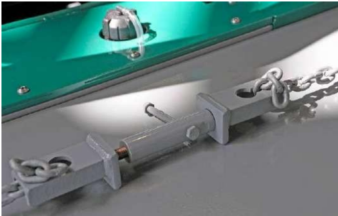
Figure 5.13 | Securing ballast plates – Prins Sprinter
