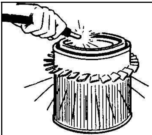
Figure 6.2 | Hose down air filter element
